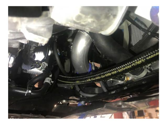
2.5 Secure the line to the radiator fan shroud frame behind the radiator as shown using zip-ties. Make sure to slide the thermo cover on the hoses near the downpipe. (not shown in the picture) (Parts used #11)
