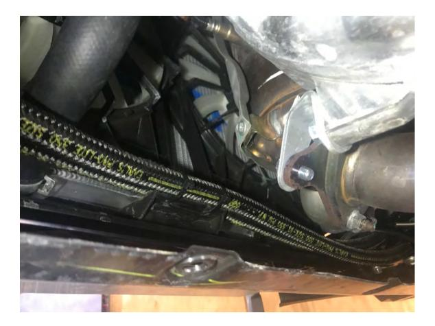
2.6 install the Air Duct Plate as shown in the picture. Secure the front top on the plate to the bumper reinforcement bar using the tapping screw provided. (Parts used #9,10)
