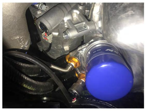
(picture shows optional pressure and temp fitting)
